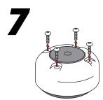
Remove the four screws using a 2.5 mm allen wrench.
