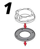
Place the plastic base onto the rubber base gasket. Be sure to line up the four screw holes.
