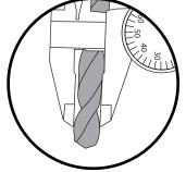
Measure your cable diameter and select the appropriate drill bit. For a 0.25" cable use a 9/32" or 7mm drill bit. For a 0.40" cable use a 7/16" or 11mm drill bit.
