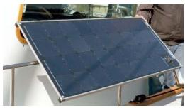
on hand rails, the clamps can be mounted on the 1 ½" Cross-Beams either on the centre-line of the panel, or to one side.
