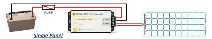
Controller must be able to handle full rated voltage and current output of the panel. Cables must able to safely handle maximum current, and be sized for 3% volt-drop. Fuse should be max current plus 50%
