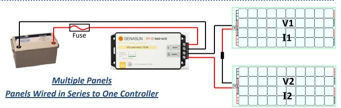
Should only be considered where shade is not anticipated, as any shading on any part of even one cell will reduce current output of the whole array proportionally. Total system voltage (Vt) will be sum of V1 and V2 (Vt =V1+V2). Total current (It) will be equal to I1 and I2 (It=I1=I2). Controller must be able to handle Vt and It. Cables must able to safely handle maximum current (It), and be sized for 3% volt-drop. Fuse should be max current plus 50%.
