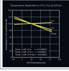
Effects of Cell Temperature on Power, Current, and Voltage
