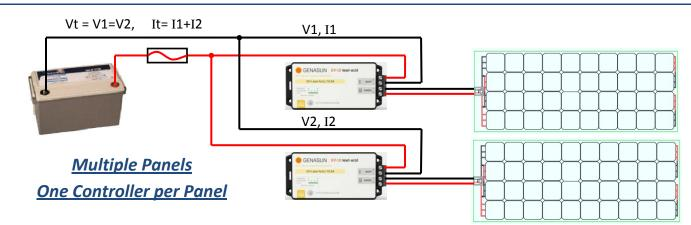
The best solution for multiple panels. Controllers must be able to handle full rated panel voltage and current output . Cables must able to safely handle maximum current, and be sized for 3% volt-drop. Fuse should be max current plus 50%.
