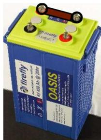
The battery will be shipped with the connection bar shown above. This connects the 2 cells inside the module in series making the battery 4V and 450Ah. For a 12V x 450Ah bank, connect 3 x 4V/450Ah in series (3S). For 24V x 450Ah, connect 6 in series (6S). For 900Ah x 12V, it must be 3S x 2P (3 batteries in series and then parallels with the other series string). For 900Ah x 24V,
