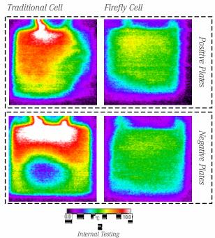
Infrared thermal images snapped at the end of a 5C (12 minute) discharge of both a Firefly 3D cell and a Traditional cell.
