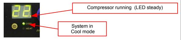
The LED indicator for the compressor can be steady or blinking: A steady LED means that the compressor is running. A blinking LED indicates that there is a timer delaying the compressor from starting. In this condition the fan and the sea water pump will be running, while the compressor is waiting the timer to expire. When the LED becomes steady, the compressor will start automatically.
