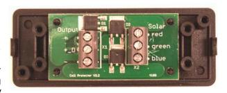
activated under total shading conditions such as a complete blockage of sunlight to one or more cells if canvas, clothing, etc. becomes draped on the panel. Under those conditions the diodes will prevent a cell(s) from burning and destroying the panel. Mount the Diode Box in a dry location, preferably within the scope of the 8' (approx.) cable provided. Contact Coastal Climate Control for options if extending the cable is deemed to be necessary or desirable.
