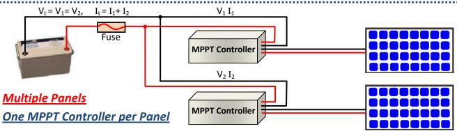
Best solution for multiple panels. MPPT Controllers must be able to handle full rated panel voltage, and maximum individual panel current output plus at least 30%. Cables must able to safely handle maximum expected current, and be sized for 3% voltdrop. Fuse size should be maximum anticipated current plus 50%.
