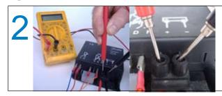
Turn the fridge off. Then using a d.c. voltmeter or a multi meter place one of the meter probes in the terminal marked + on the Danfoss controller and place the second meter probe in the terminal marked - on the Danfoss controller and read the voltage.
