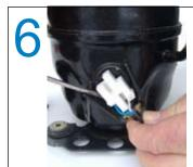
Carefully remove the plug from the compressor. It may be nessecary to use a small screwdriver to lever the plug from the compressor, if so try to move each side of the plug alternately by only 1 or 2 millimetres each time.
