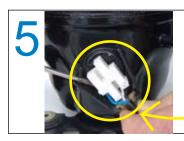
Take note of the orientation of the plug on the compressor so you can replace it correctly.
