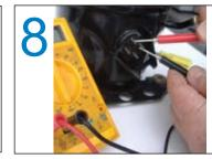
On your meter select the lowest range capable of measuring 5 ohms. Place one meter probe on pin 3. Place the second meter probe on pin 1, then pin 4, then pin 2, recording the values for each.
