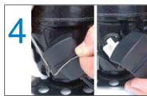
Remove the metal clip and plastic cover from the compressor plug. You may need to lever it off with a screwdriver.
