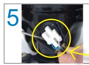
Take note of the orientation of the plug on the compressor so you can replace it correctly.
