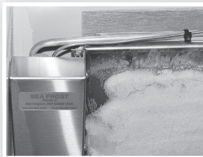
The Sea Frost features a stainless-steel evaporator plate (above left) built for durability. Though better at transferring heat, aluminum plates tend to wear out in eight to 10 years.
