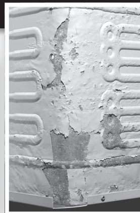
The Sea Frost features a stainless-steel evaporator plate (above left) built for durability. Though better at transferring heat, aluminum plates tend to wear out in eight to 10 years.
